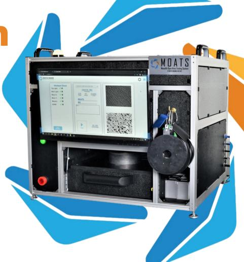
The Monolith Open Area Testing System (MOATS) is an advanced, high-precision imaging solution designed specifically for the inspection and analysis of coated and uncoated monoliths in industrial applications.
